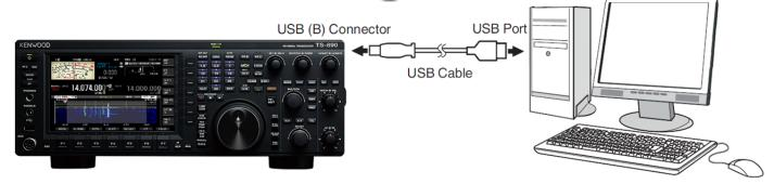
The KENWOOD TS-890S is equipped with a USB (B) connector for exchanging both of audio signals and PC control commands for performing data communication with an external device such as a PC.
